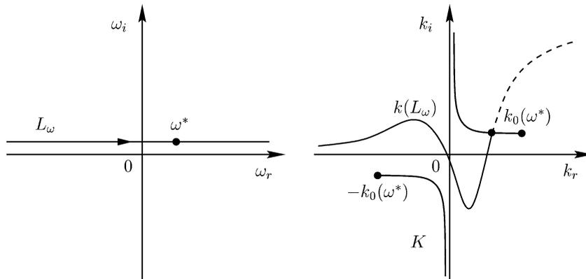
Fig. 1. Locus of spatial branch in complex  $k$ -plane as  $\omega$  moves along  $L_\omega$  contour in complex  $\omega$ -plane for small  $\omega_i$ . The branch cut  $K$  for the function  $\lambda$  join the critical points for  $\omega = \omega^*$ . Dashed line: analytic continuation into the second sheet of the Riemann surface (corresponding to solutions which become exponentially large as  $r \rightarrow \infty$ ).
