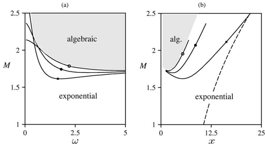
Fig. 6. Domain of exponential-algebraic transition in  $M$ - $\omega$  (a) and  $M$ - $x$  (b) planes for non-axisymmetric modes.  $\blacksquare$ ,  $n = 1$ ;  $\bullet$ ,  $n = 2$ ;  $\circ$ ,  $n = 3$ ; the dashed line in (b) gives the end of the core region.
