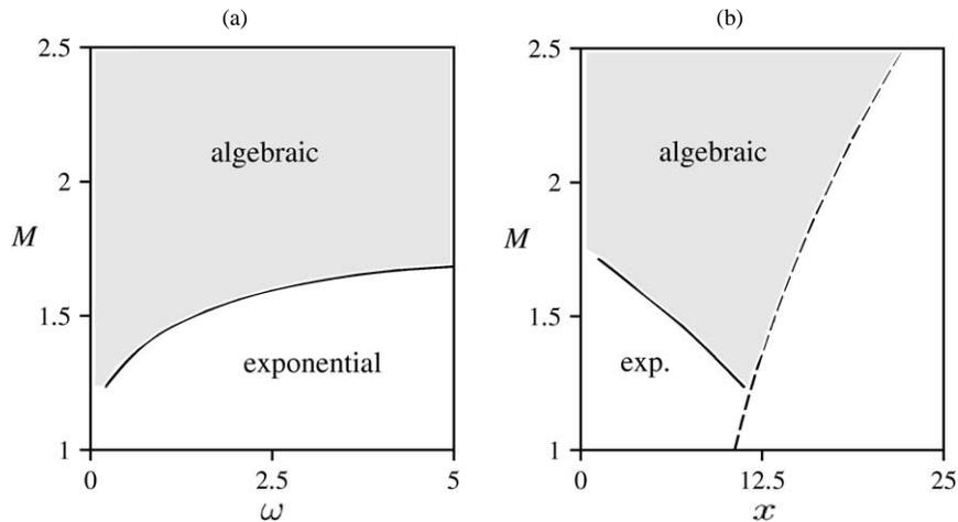
Fig. 5. Domain of exponential-algebraic transition in  $M$ - $\omega$  (a) and  $M$ - $x$  (b) planes for  $n = 0$ . The dashed line in (b) gives the end of the core region. For each point located above the curve, into the grey domain, the cross-stream decay is algebraic at a location corresponding to the stationary phase point of the pressure far-field.
